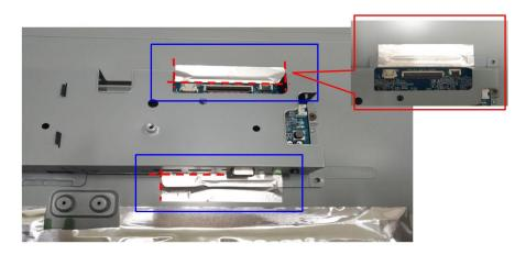
Step5. Insert 10 pin back light WH to panel and main board, use acetate tape to fix. (Tape in red circle).
