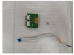
Step.11 Unscrew two screws and disassemble key board from rear cover and separate navi key& cable
