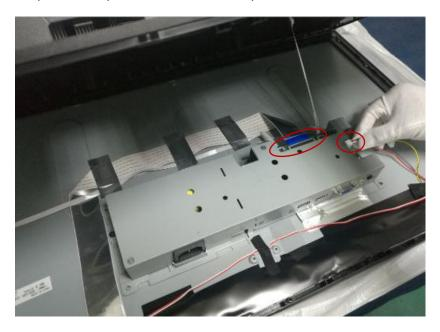
Step.5 Unscrew screws on main shielding and disassemble AL tape
