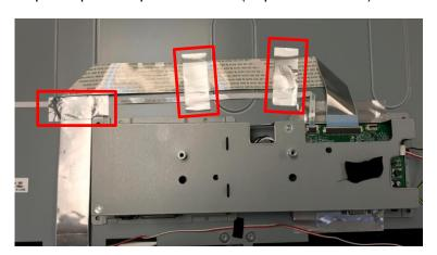
Step8. Assembly middle frame with LCM and fix screw (in red circle)
