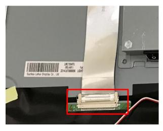
Step3. Lock the shielding on panel with screw. (in red circle)
