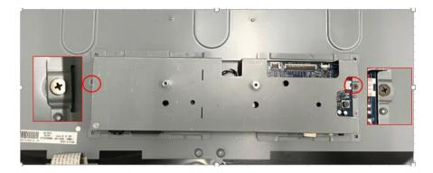
Step4. Use Al tape to fix shielding (tape in blue circle).
