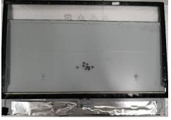
Step.9 Separate gasket and lens from MID frame
