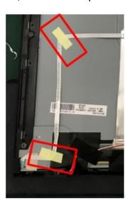
Step6. Insert 10 pin back light FFC and 30 pin LVDS FFC to main board. Use yellow tape to fix.
