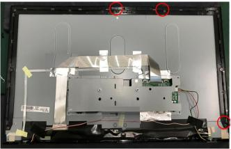
Step10. If with speaker model, assembly speaker on middle frame, and assembly speaker cable on main board. (red and white cable is on left side, yellow and black is on right side.)
