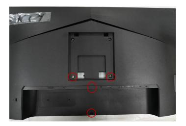
Step.3 Separate hooks between MID\_FRAME and R/C
