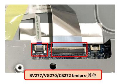
Step7. Tape AL tape to fix FFC. (Tape in red circle).
