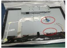
Step.6 Separate speaker from MID\_FRAME and LVDS & Backlight FFC from LCM
