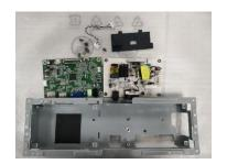
Step.8 Unscrew eleven screws and separate MID FRAME and LCM
