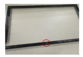
Step.10 Unscrew one screw and disassemble USB board from rear cover and separate USB & cable
