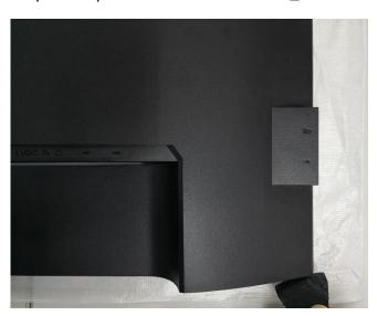
Step 4. Pull up the Rear Cover and pull out all connectors
